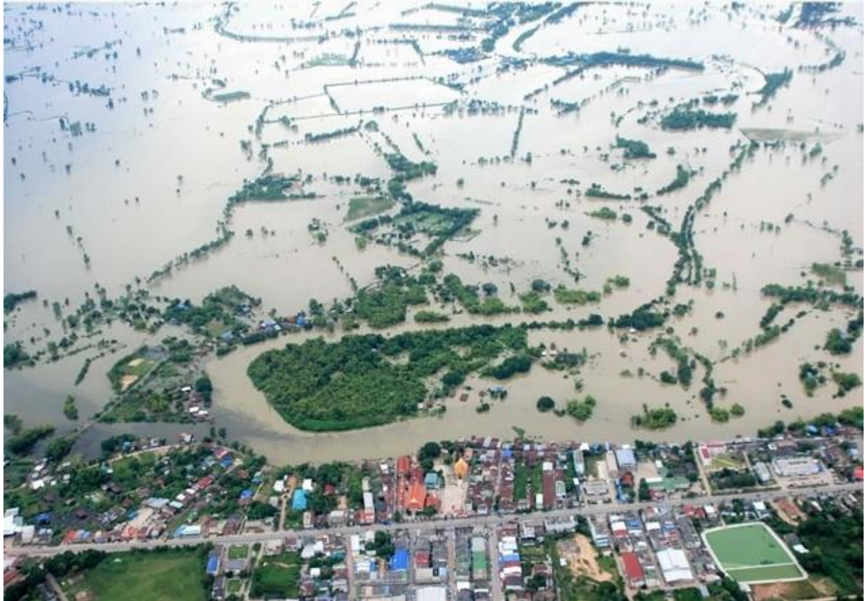
Flood retention areas in the Bang Rakam model prevent flooding along the Yom river from overflowing agricultural zones in the wet season (photo credit: Thai-German Climate Programme – Water )
