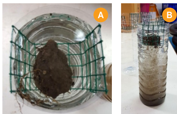
Fig. 2.2 Place an air-dried soil clod sample in a wire mesh basket (A), after water absorption, aggregates inside the clod are forced by water to break apart and small soil particles sink to the bottom of the container (B).
