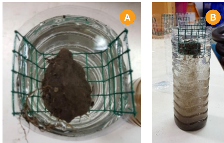
Fig. 2.1 Place an air-dried soil clod sample in a wire mesh basket (A), after water absorption, aggregates inside the clod are forced by water to break apart and small soil particles sink to the bottom of the container (B).
