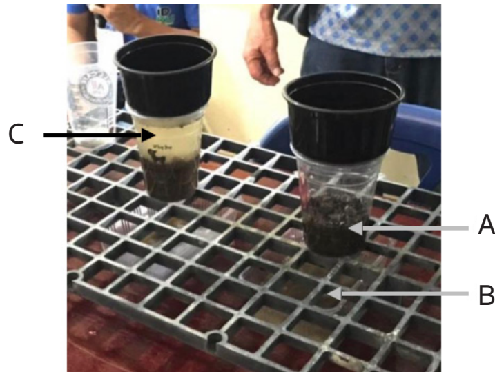
Fig. 2.2 Comparison of infiltration rate between soils of different aggregate stability. Healthy soil sample holds water evenly (A) and drained excess water out into a container (B). Infiltration of common soil is very slow, retaining water above soil surface (C).
